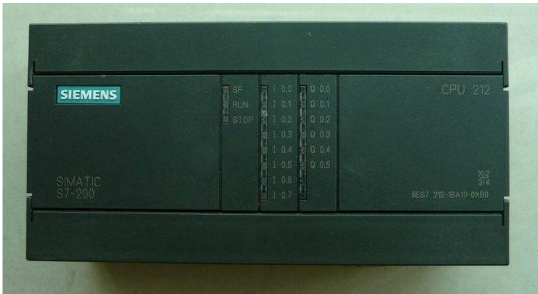
Figure11. PLC.Model No. 6ES7212-1BA10-0XB0, SIMATIC S7-200, CPU 212
